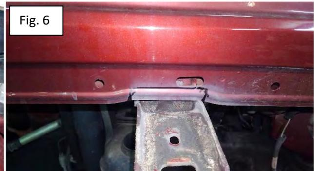
10. Observe the front edge of the cowl and note that there are ribs present in the center of the front lip. These ribs help give the cowl a slight arch in the center. Use a pair of pliers to carefully flatten out these ribs, which in turn will flatten the top of the cowl and remove the arch present in it.
